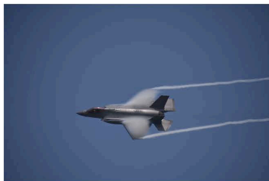
F-35 pulling streamers from the wing tips in a high-G turn. What appears to be an out-of-focus photo is actually water vapor formed above the wing demonstrating the Bernoulli effect.
