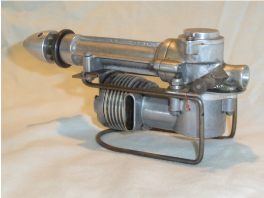
Lee Sidewinder Version I. This engine is one of three of this version to be hand built by Clarence Lee. Note the sheet metal mounting lugs and side facing exhaust port.
