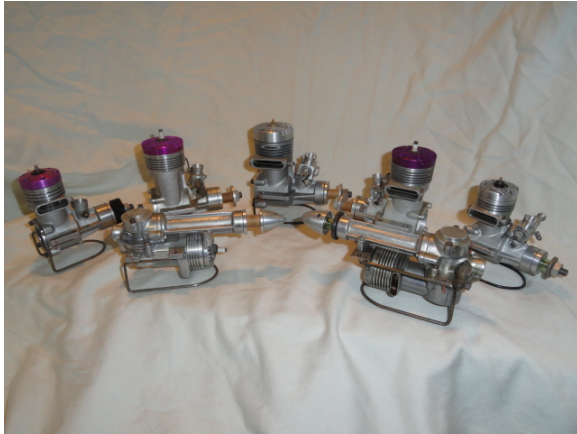
Group image of the Lee series of engines. Foreground left Sidewinder Version II, foreground right Sidewinder Version I, background starting on the left Veco .35, Lee .51, Veco .61, Lee .45, Veco .19).
